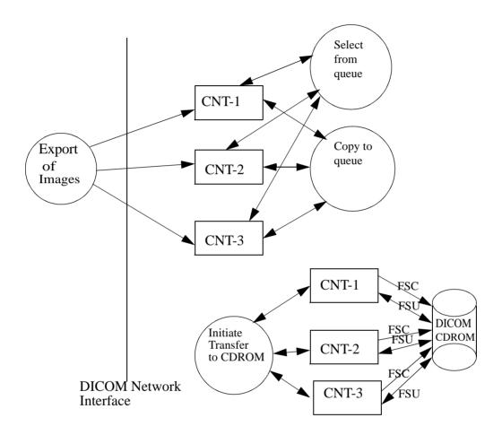
The Inturis DICOM Recorder can receive DICOM XA and SC images over the network. All images received in *one* DICOM association and belonging to the same patient are combined in *one* entry in the queue of the recording station. Afterwards, the operator can select the entries for inclusion on a DICOM CDROM.
